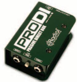
*The Radial ProDI is a passive direct box that combines exceptional audio performance with solid dependable construction, making it the ideal general duty direct box for stage and studio.*
