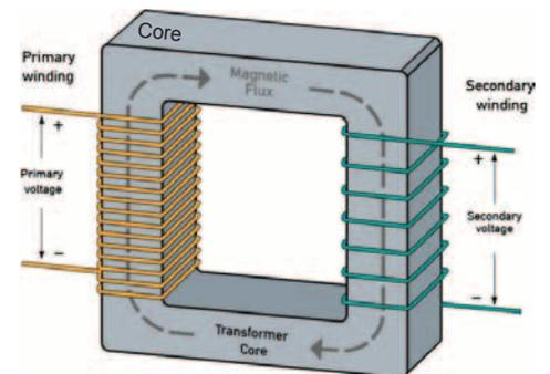
*Unlike solid state circuits, transformers 'gradually' saturate when pushed hard.*
